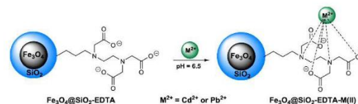
Fig. 5. Scheme of proposed mechanism of Cd(II) and Pb(II) ions binding by Fe 3 O 4 @SiO 2 -EDTA nanoparticles.
