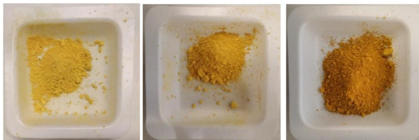
Fig. S3 Distinguishable color change of prepared ZIS/CIS-7, ZIS/CIS-10.5 and ZIS/CIS-12.5 samples from left to right
